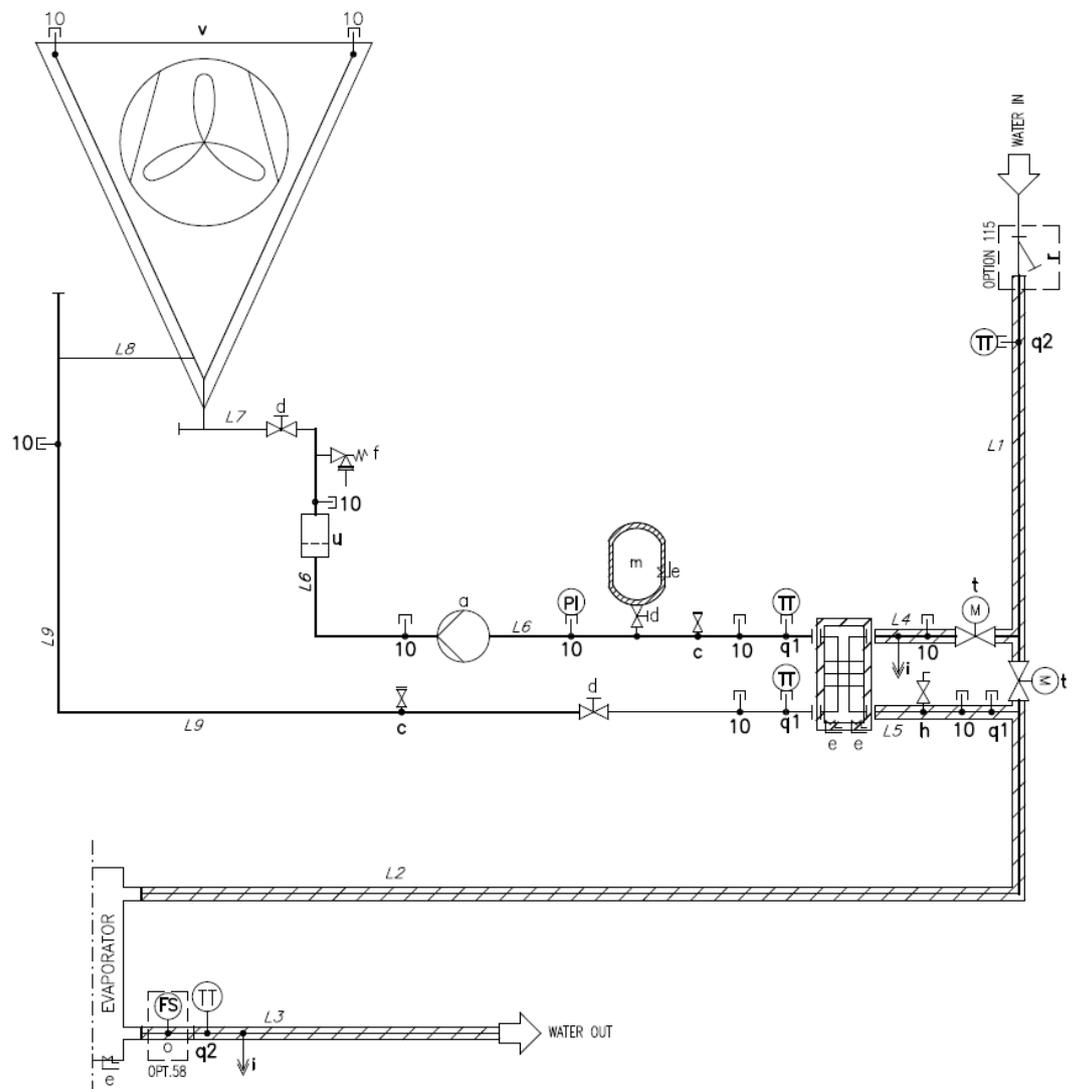
**Fig. 21– Circuito fechado Hydronic Free cooling P&ID (Opt. 231)**
