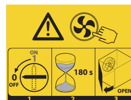
Danger of running fans
