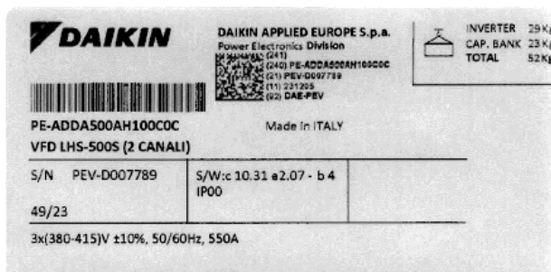
Fig.° 14– VFD LHS Identification Label
