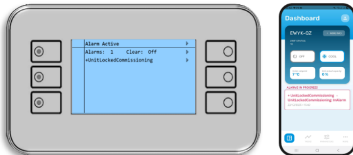
POL 871 and Daikin Map with commissioning alarm
